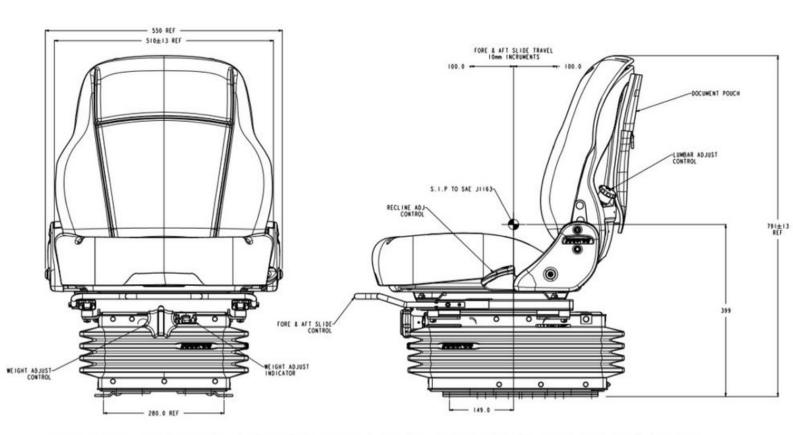
HEAVY DUTY MECHANICAL SUSPENSION WITH 3 STAGE HEIGHT ADJUSTMENT AND DUO DAMPER
