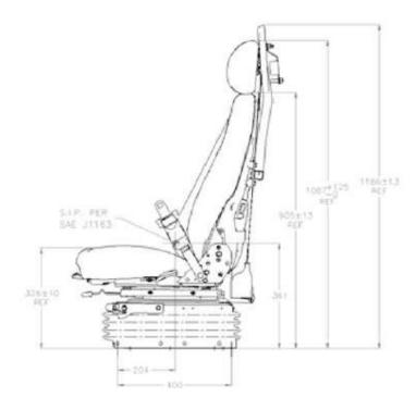
Wide Severe duty Toggle Link low frequency air suspension, adjustable damper and Airide high volume air spring. 220KG weight rated suspension assembly available in 24 volt compressor or straight air feed configurations.
