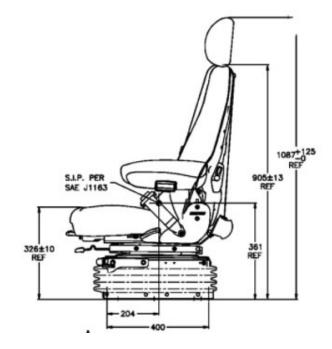
Wide Severe duty Toggle Link low frequency air suspension, adjustable damper and Airide high volume air spring. 220KG weight rated suspension assembly available in 24 volt compressor or straight air feed configurations.
