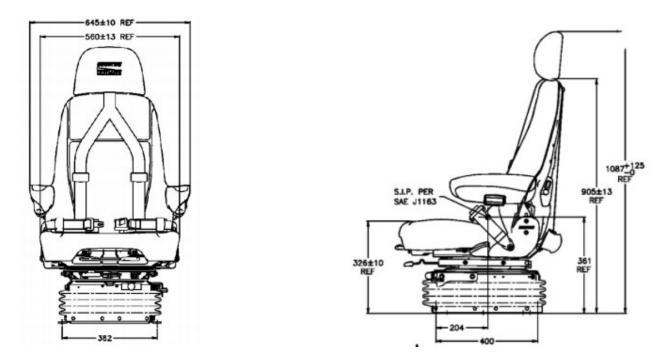
Wide Severe duty Toggle Link low frequency air suspension, adjustable damper and Airide high volume air spring. 220KG weight rated suspension assembly available in 24 volt compressor or straight air feed configurations.
