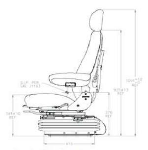
Heavy Duty 24V air suspension with Airide® high volume air spring & double acting adjustable Duo® damper.
