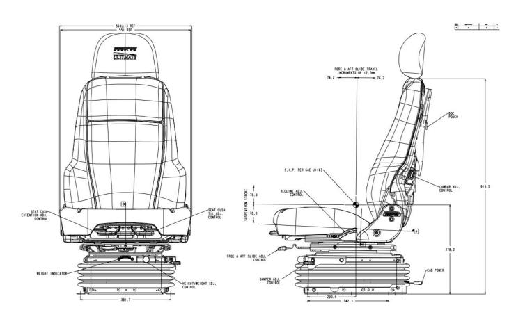
Comes with OEM KOMATSU 24V or optional Straight Air Suspension (no internal air compressor) with Airide® high volume air spring and double acting Duo®Damper. Suits WA Loader Series, GD Grader Series, 830 – 930 & HD & HM Truck Series
