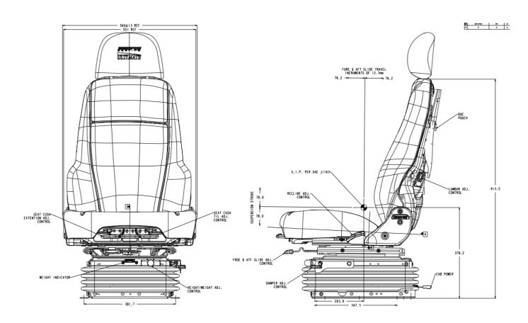
Comes with OEM **CATERPILLAR** 24V or optional Straight Air Suspension (no internal air compressor) with Airide® high volume air spring and double acting Duo®Damper. Direct fit for all CAT OFF HIGHWAY TRUCK, D400E, 700 Series Articulated, MOXY, BELL, Hitachi, VOLVO, TEREX, KOMATSU and a wide variety of applications in Mining, Forklift, Construction, Agricultural and many other industries.
