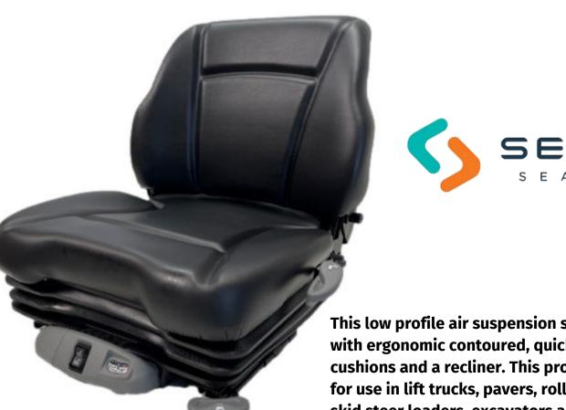
This low profile air suspension seat is engineered with ergonomic contoured, quick-release, comfort cushions and a recliner. This product is designed for use in lift trucks, pavers, rollers, mini dumpers, skid steer loaders, excavators and other compact machines and is available in a variety of trims and colours.
